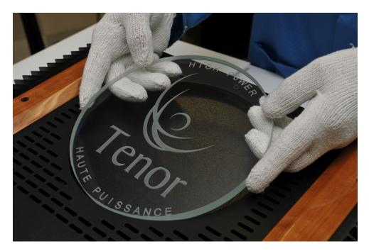
B. Carefully lower Starfire Crystal by transferring grip slowly and surely to sides of Crystal as shown below:
