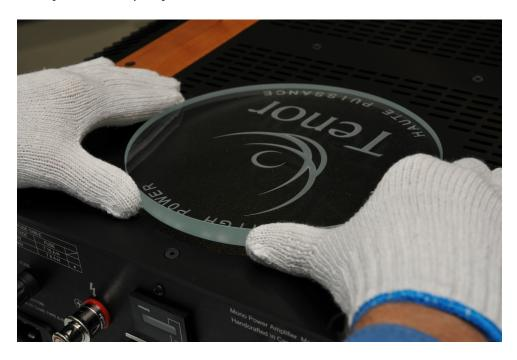
C. Once Starfire Crystal is set in position carefully rotate until the logo is aligned with the amplifier top and the Crystal has equal space all around it:
