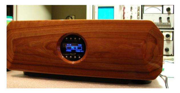
Vacuum Florescent Display mounted in cherry wood front panel with buttons above/below display for on/off/selections/programming.
